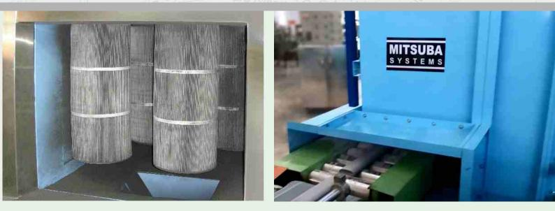
Mitsuba offers Dusting unit for spraying Chalk / Talc powder on Green Rubber Tubes used in Automobile industry.
